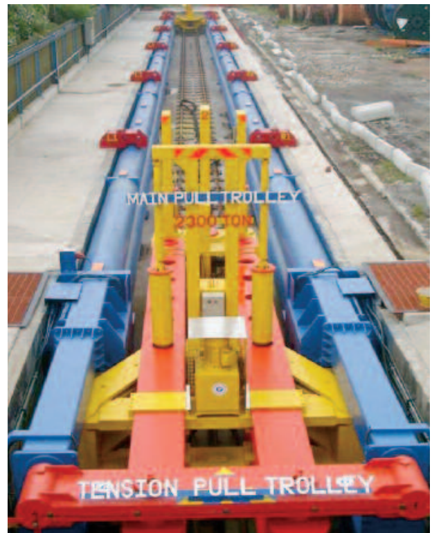
Franklin 2,300 Tonne Hydraulic Test Bed
