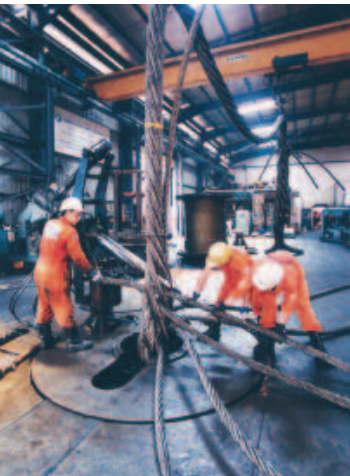
Manufacturing Franklin Cable Laid Slings
