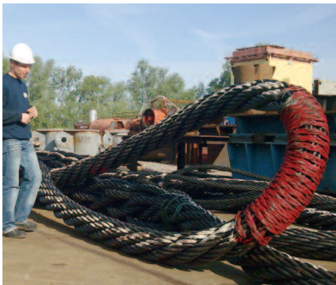
Clients' slings for refurbishment
