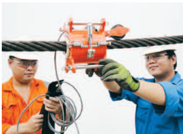
Calibration E- Mag unit on test rope
